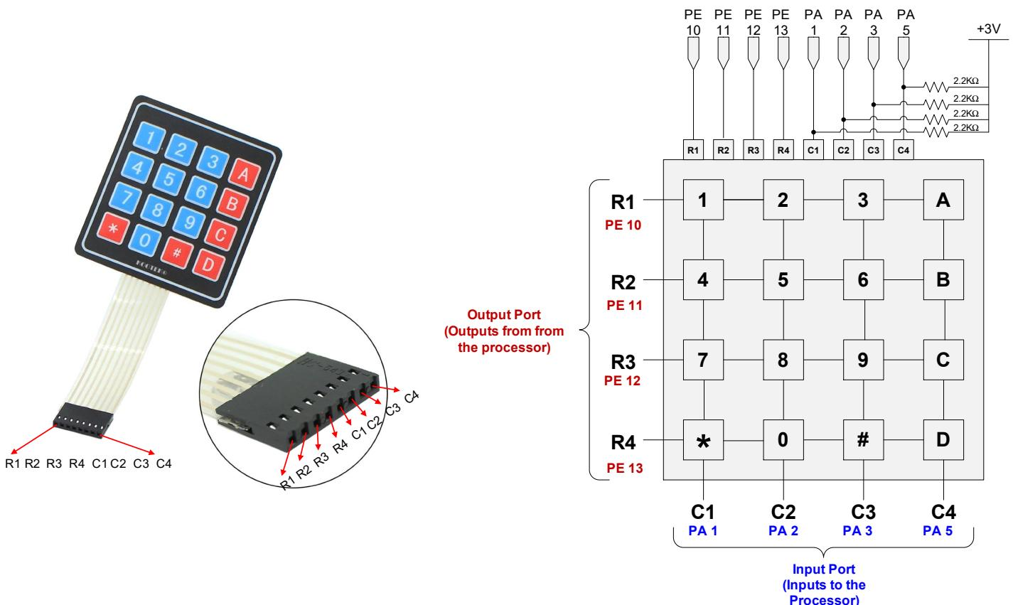
The maximum current a GPIO pin can source or sink is 20 mA. When calculating the value of external pull-up resistors, make sure that the current should not exceed 20 mA.
