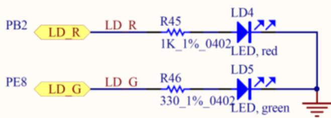
Consider that our final objective is to turn on the **green LED** in our Discovery kit located on pin **PE.8**. You are required to write a bit of C code in each of the questions below in order to achieve this objective.
