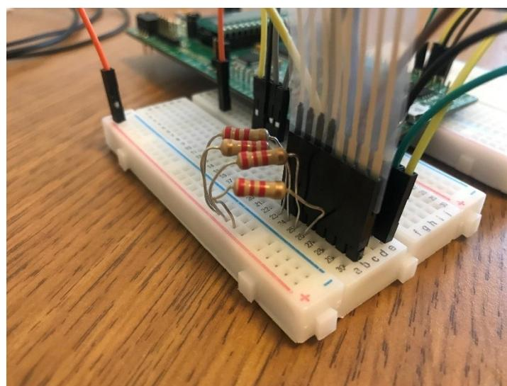
On the STM32L4 board, all pins in the input port (PA0, PA1, PA2, PA3, and PA5) are connected to ground via a 100nF capacitor, as shown in the figure below. Therefore, due to these capacitors, the voltage output on these pins won't immediately change to Vcc or ground. **A very short delay should be added before reading the input port.** Specifically, delays are needed between setting GPIOE outputs and reading GPIOA inputs.
